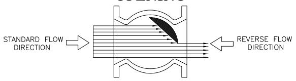
Upon opening the valve, the initial rotation of the plug causes the resilient seating surface to move axially away from the nickel seat in the body. This action minimizes wear and scraping of the resilient seat, thereby improving the life of the valve. The plug can be positioned at any position between open and closed for throttling applications.
