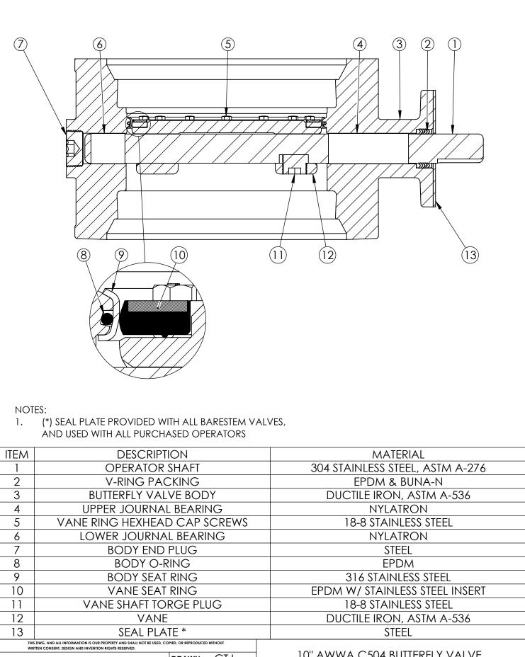
M&H VALVE COMPANY A DIVISION OF MC WANE INC. P.O. BOX 2088 ANNISTON, ALBAANA 36202 DRAWN: CTJ DATE: 4/8/2021 DWG. NO. BB10-M33-B0000-11110 10" AWWA C504 BUTTERFLY VALVE MECHANICAL JOINTS - RATED CL250 BODY SUB-ASM MATERIAL LIST FA12 OPERATOR FLANGE
