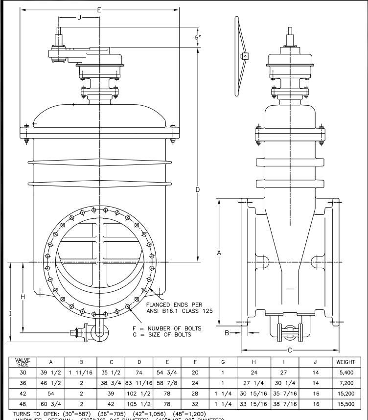
HANDWHEEL OPTIONAL: (30"&36"=24" DIAMETER) (42"&48"=28" DIAMETER)
